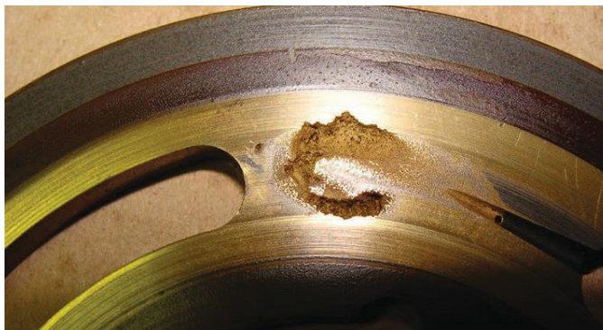
Cavitation wear and microdieseling damage. (Photos courtesy of Hegelsen Industries in Hartford, Wis., and Milwaukee School of Engineering.)
